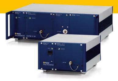
PSS spectrometers offer an optimal solution for NIR process analytics. Based on diode array technology combined with superior transmission grating design, PSS spectrometers are used for fast and reliable data acquisition. The use of fiber coupled probes enables flexible integration in various measurement scenarios.
